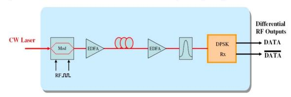
The integrated DPSK receiver combines a delay-line interferometer (DLI) with a balanced receiver to achieve compact size in a butterfly package. Compared with discrete components, the integrated receiver couples optical outputs from the DLI directly into the balanced photodetectors, resulting in smaller insertion loss and low channel skew, in addition to the elimination of fiber routing and matching.
